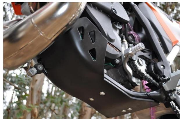
**Engine Guard DTC-EC**
